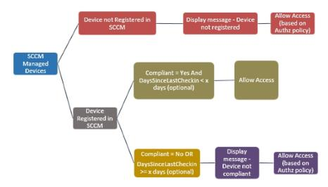
When a device connects to the network and a Microsoft SCCM policy matches, Cisco ISE queries the relevant SCCM server to retrieve compliance and last login (check-in) time. With this information, Cisco ISE updates the compliance status and the lastCheckinTimeStamp of the device in the **Endpoint** list.
