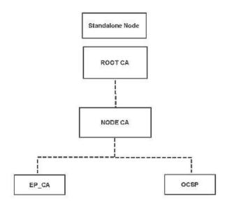
When you set up a deployment, the node that you designate as the Primary Administration Node (PAN) becomes the Root CA. The PAN has a Root CA certificate and a Node CA certificate that is signed by the Root CA.
