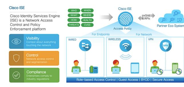
Cisco Identity Services Engine (ISE) is an identity-based network access control and policy enforcement system. It functions as a common policy engine that enables endpoint access control and network device administration for enterprises.
