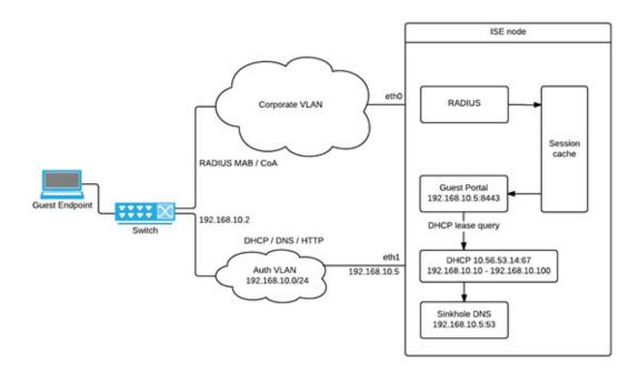
The following diagram displays a network with Auth VLAN and an IP helper.
