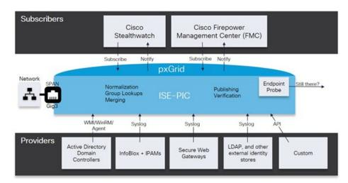
Subscribers connected to Cisco ISE must register to use the pxGrid services. Subscribers should adopt the pxGrid Client Library available from Cisco through the pxGrid SDK to become the clients. A subscriber can log in to pxGrid using a unique name and certificate-based mutual authentication. Once they have sent a valid certificate, Cisco pxGrid subscribers are automatically approved by ISE.
