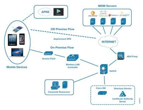
Figure 30: MDM Interoperability with Cisco ISE
