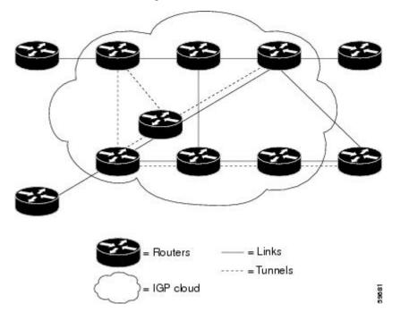
As a result, a TE tunnel is advertised as a link in an IGP network with the link's cost associated with it.
