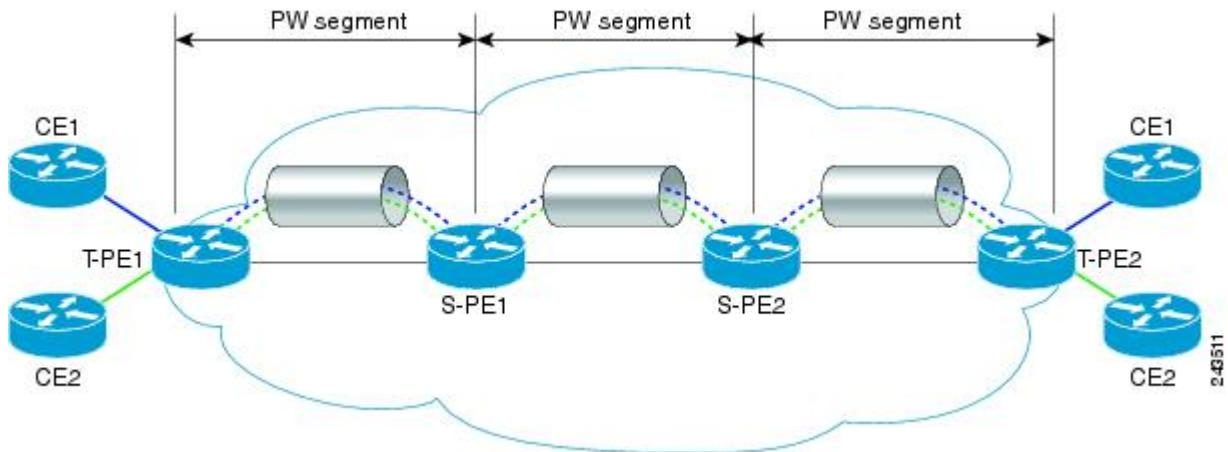
The end routers are called terminating PE routers (T-PEs), and the switching routers are called S-PE routers. The S-PE router terminates the tunnels of the preceding and succeeding PW segments in an MS-PW. The S-PE router can switch the control and data planes of the preceding and succeeding PW segments of the MS-PW. An MS-PW is declared to be up when all the single-segment PWs are up. For more information, see the *L2VPN Pseudowire Switching* document.
