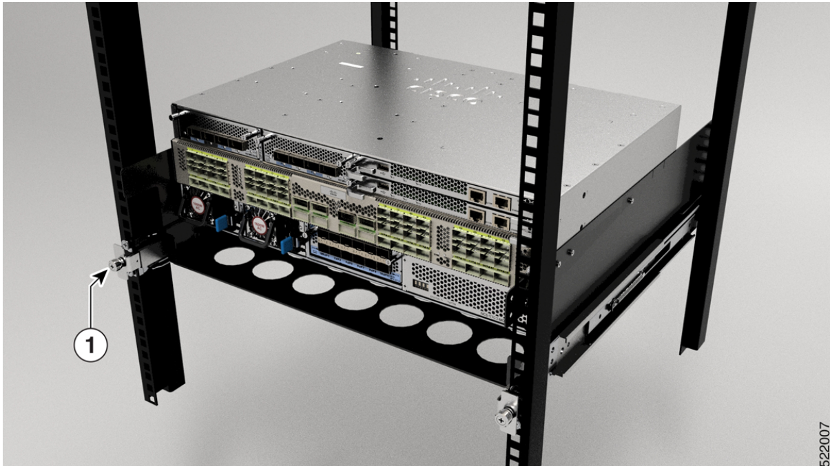
Figure 69: Secure the Tray to the Rack
