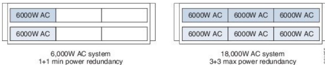
Figure 94: AC System Power Redundancy for the Cisco ASR 9010 Router—Version 3
