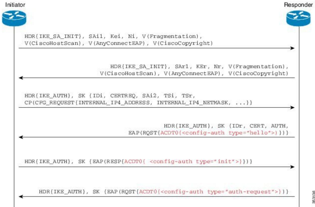
1. Cisco AnyConnect client initiates IKE connection to FlexVPN server. The client sends vendor ID payloads to indicate support for Cisco AnyConnect EAP in addition to the typical IKE payloads. The client identifies itself as a Cisco product by including the Cisco copyright vendor ID.
