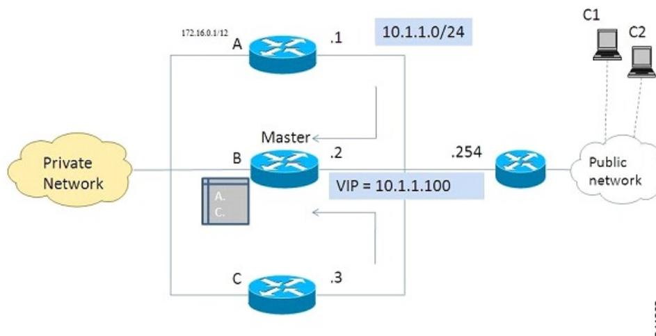
1. An active HSRP gateway is elected as “primary” in the HSRP group and takes ownership of the Virtual IP address (VIP) for the group. The primary maintains a list of gateways in the cluster, keeps track of the load on each gateway, and redirects the FlexVPN client requests to the LLG.
