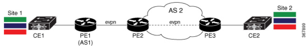
Figure 55: BGP over MPLS (Inter AS)
