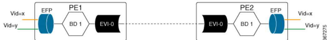
Figure 53: VLAN Bundle Service Interface
