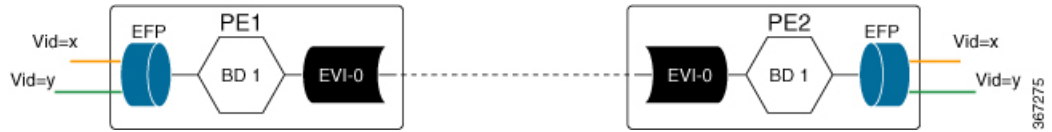
Figure 47: VLAN Bundle Service Interface
