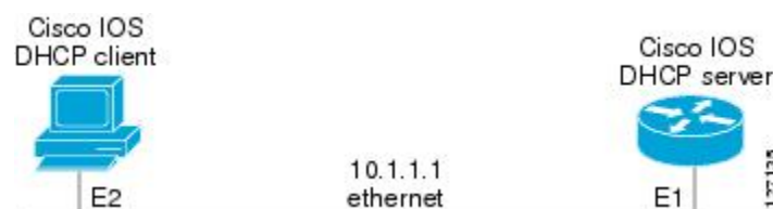
Figure 10: Topology Showing DHCP Client with GigabitEthernet Interface
