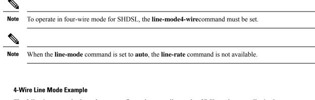
The following example shows how to configure the controller mode of DSL on the controller in slot 4 and port 0 to operate in four-wire mode:
