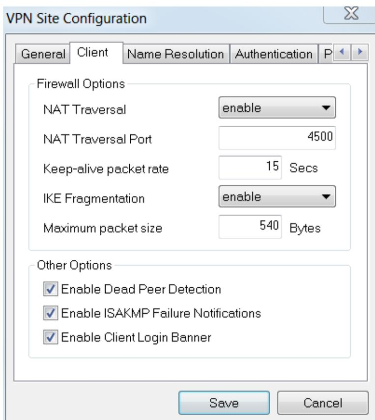
The screenshot shows the "VPN Site Configuration" dialog box with the "Client" tab selected. The "Firewall Options" section includes:
