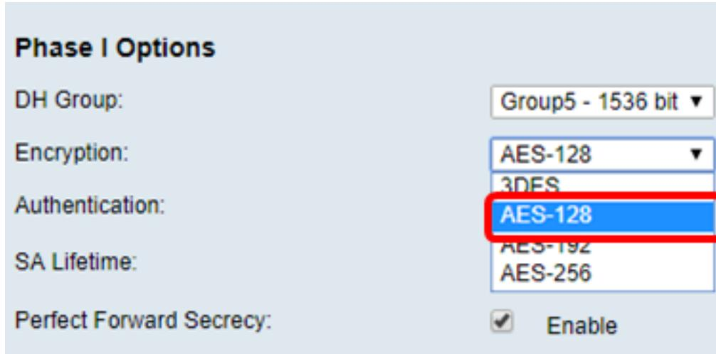
The screenshot shows the 'Phase I Options' configuration window. The 'DH Group' is set to 'Group5 - 1536 bit'. The 'Encryption' dropdown menu is open, showing options: AES-128, 3DES, AES-128 (highlighted with a red box), AES-192, and AES-256. The 'Authentication' field is empty. The 'SA Lifetime' field is empty. The 'Perfect Forward Secrecy' checkbox is checked and labeled 'Enable'.
