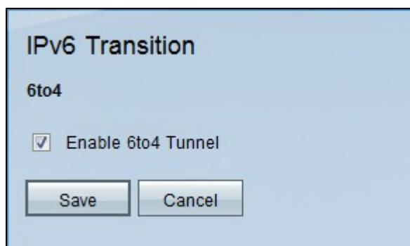
Enable 6to4 Tunneling on IPv6 and IPv4 interfaces.
