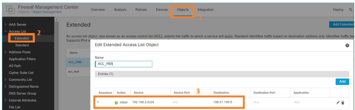
The screenshot shows the 'Objects / Object Management' section of the Firewall Management Center. The 'Objects' tab is selected (1). In the left sidebar, 'Access List' is expanded (2), and 'Extended' is selected. The main panel displays the 'Extended' access list object 'ACL\_PBR'. It includes a table with one entry:
