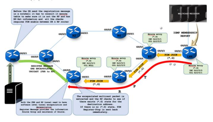
The RP also sees that an active shared tree with a nonempty outgoing interface list exists and therefore sends the deencapsulated packet down the shared tree.
