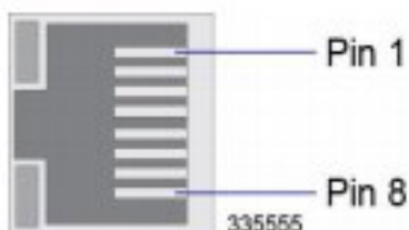
Figure 31. SPIO Ethernet RJ-45 Interface
