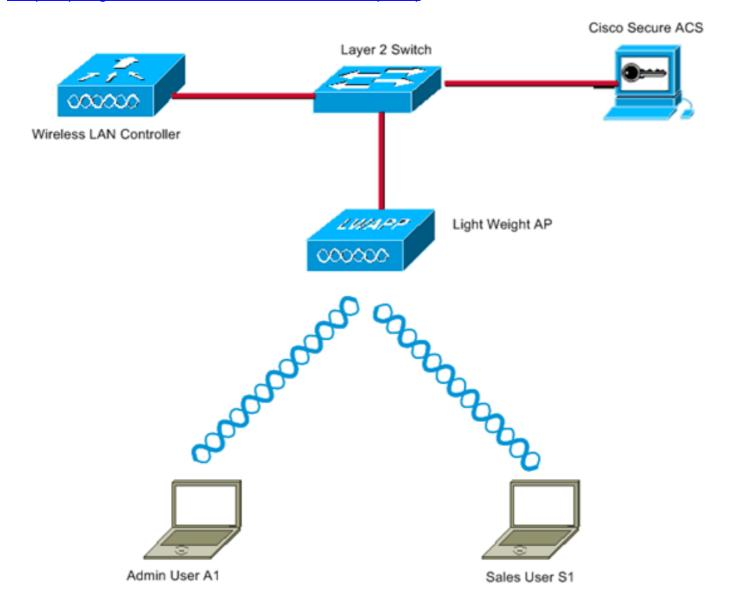
WLC Management Interface IP address: 172.16.1.30/16 WLC AP-Manager Interface IP address: 172.16.1.31/16 Cisco Secure ACS server IP address: 172.16.1.60/16
