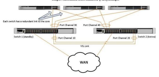
Simple Multichassis EtherChannel® (MEC) Example
