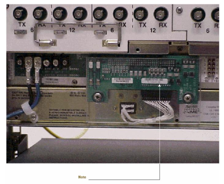
If the part number is 67-11-00015 then the AIP board needs to be replaced before the software upgrade, Any other part number on the AIP board will support both the release 2.2.2 and 3.0 software upgrades
