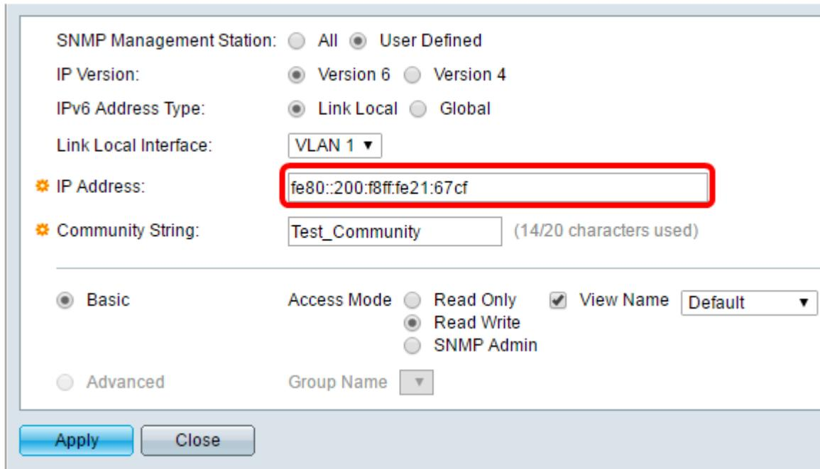
The image shows a configuration window for an SNMP Management Station. The 'IP Address' field is highlighted with a red rectangle and contains the value 'fe80::200:f8ff:fe21:67cf'. Other fields include 'Community String' with 'Test\_Community', 'Access Mode' with 'Read Write' selected, and 'View Name' with 'Default' selected. The 'Basic' radio button is selected under the mode options.
