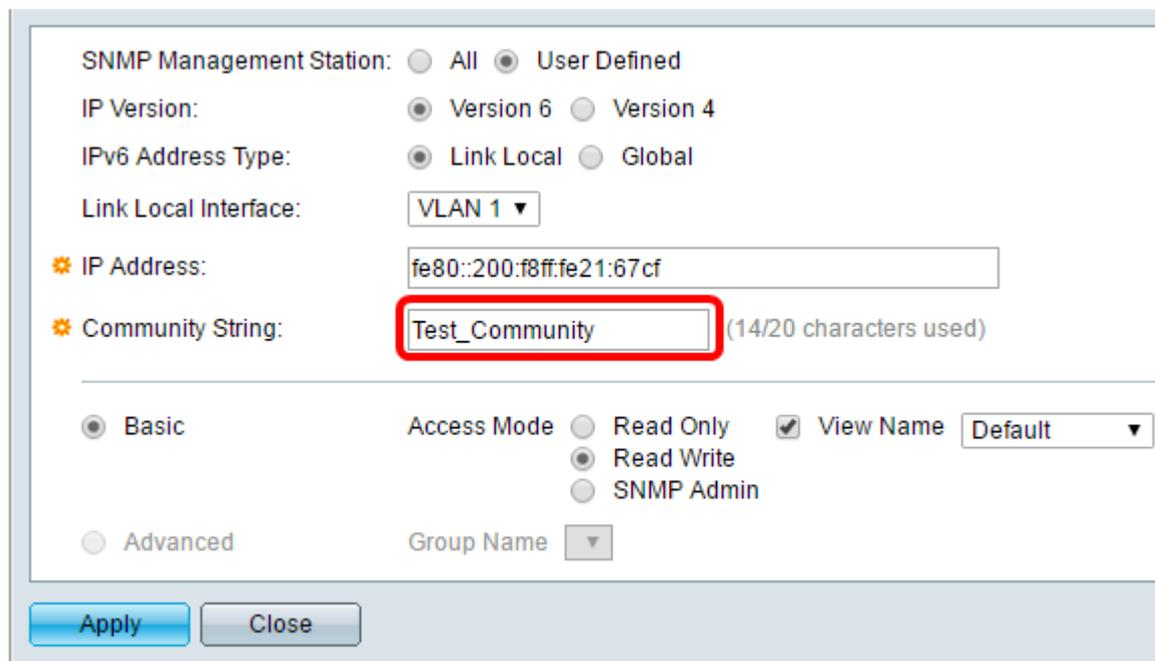
The image shows the same configuration window as above, but now the 'Community String' field is highlighted with a red rectangle and contains the value 'Test\_Community'. The 'IP Address' field is no longer highlighted.
