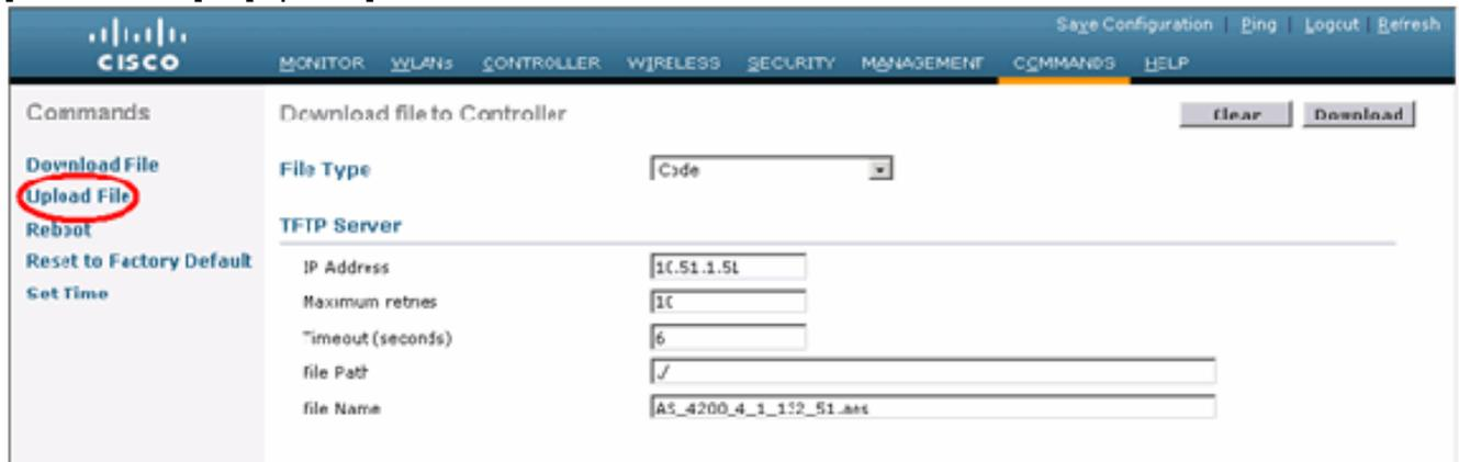
The screenshot shows the Cisco Controller GUI. The 'Commands' menu is open, and the 'Upload File' option is highlighted with a red circle. The main content area shows the 'Download file to Controller' form, which includes fields for 'File Type' (set to 'Code'), 'TFTP Server' (IP Address: 10.51.1.51, Maximum retries: 10, Timeout (seconds): 6), 'file Path' (/), and 'file Name' (AS\_4200\_4\_1\_152\_51.exe). There are 'Clear' and 'Download' buttons at the top right of the form.
