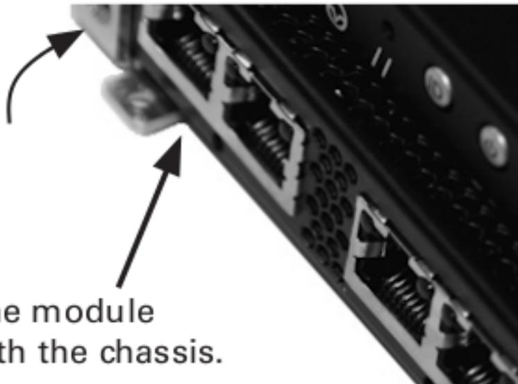
The lever is fully against the module and the module is flush with the chassis.
