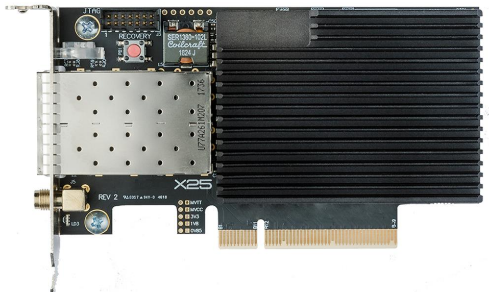
図 1 Cisco Nexus K3P-S FPGA SmartNIC
