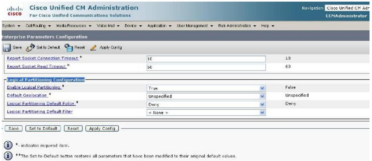
The screenshot displays the Cisco Unified CM Administration interface for Enterprise Parameters Configuration. The 'Logical Partitioning Configuration' section is highlighted, showing the following settings:
