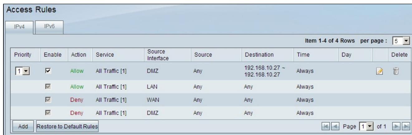
The screenshot shows the 'Access Rules' configuration window. It has tabs for 'IPv4' and 'IPv6'. The table below lists the rules:
