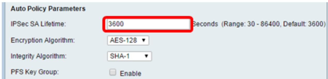
The screenshot shows the 'Auto Policy Parameters' configuration panel. The 'IPSec SA Lifetime' field is set to '3600' and is highlighted with a red border. The 'Encryption Algorithm' is set to 'AES-128', the 'Integrity Algorithm' is set to 'SHA-1', and the 'PFS Key Group' checkbox is checked and labeled 'Enable'. The text 'Seconds (Range: 30 - 86400, Default: 3600)' is visible next to the lifetime field.
