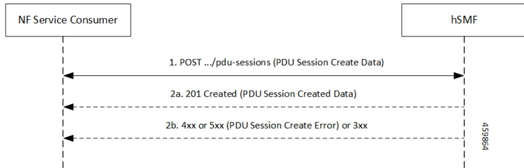
Figure 166: Create Service Operation on hSMF Call Flow
