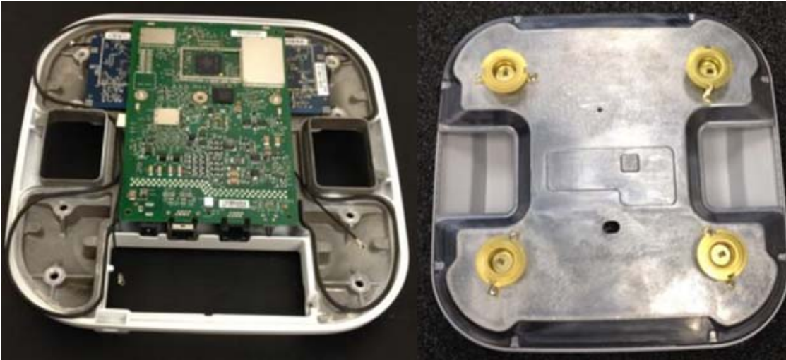
Figure 78 A Peek Inside the AP 3700 Showing Conductive Gasket and Dual-Band Antenna Design
