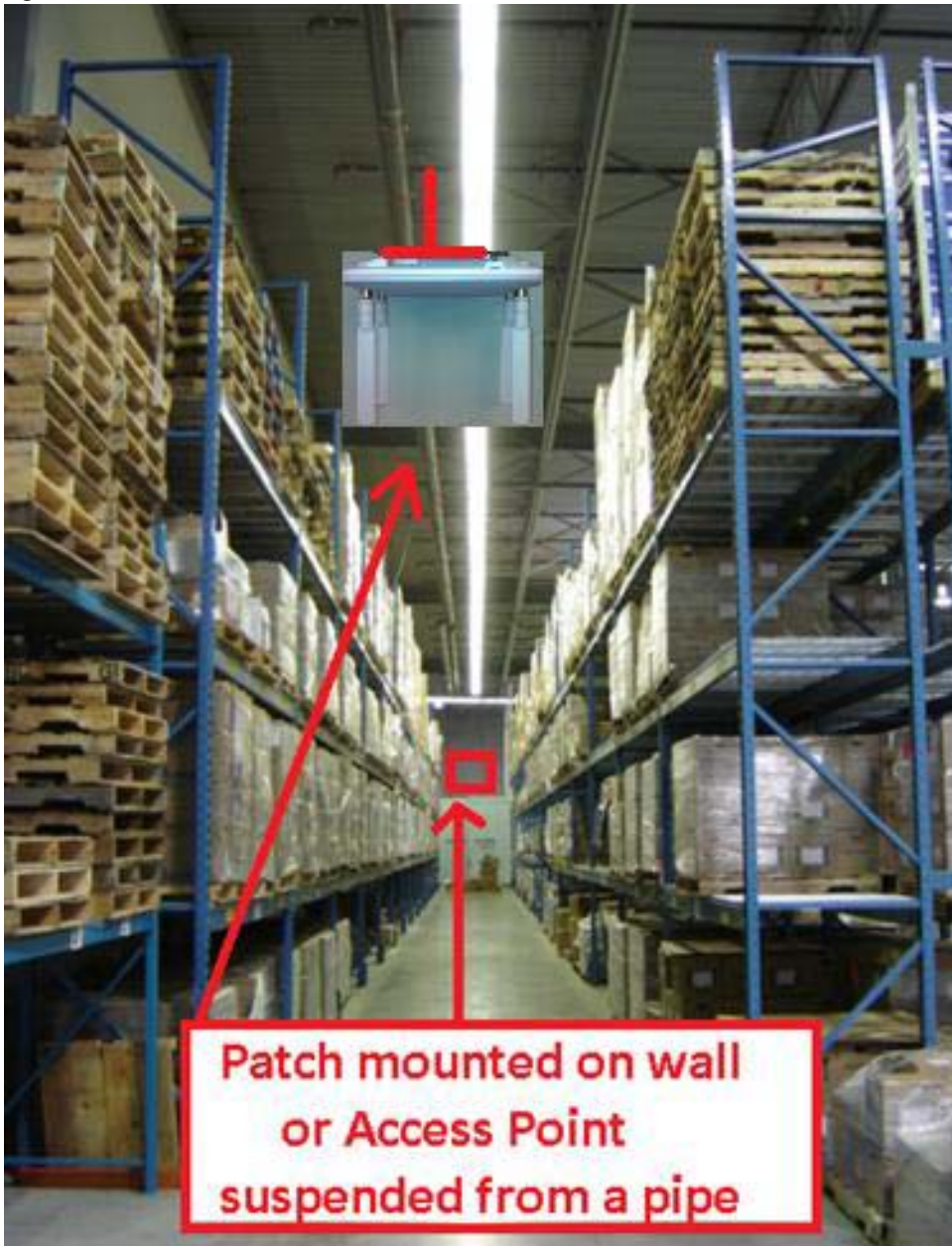
Figure 25 AP Placement in a Warehouse Environment
