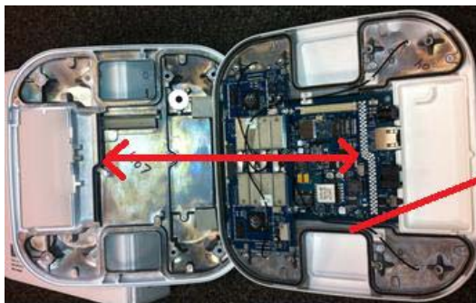
Figure 19 Inside the AP 3600 - Cover Removed (No Vents or Fans, Everything is Industrial Quality)
