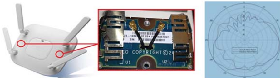
AP-3600e antenna system with module The Radio module has three internal antennas Note: AP-3600e when using directional antennas .11ac clients remain Omni-Directional
