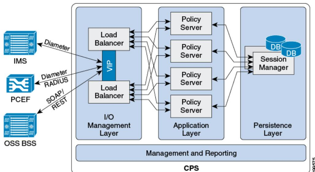
The three-tier architecture defines how CPS handles network messages and gives CPS the ability to scale. The three processing tiers are:
