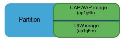
You need to choose the image to boot up with according to the mode your AP is runnning, CAPWAP or URWB. The following table provides the software images of each mode:
