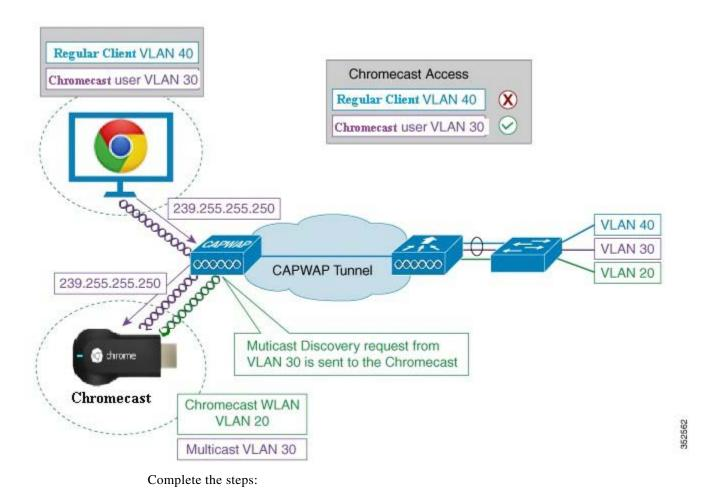
Step 1 Go to the Controller tab > Interfaces on the left-hand menu. Create the necessary interfaces for the client VLANs (student and teacher in this example) and also an interface for the Chromecast subnet (chromecast\_device in this example).
