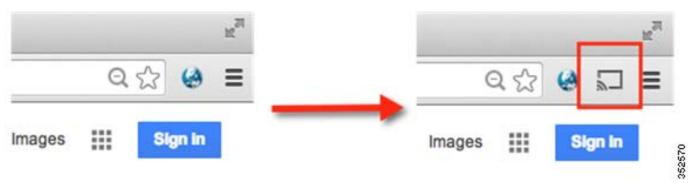
Step 4 Make sure that the Computer is connected to the client wireless network and gets an IP address from the Teacher VLAN. Click the googlecast tab on the teacher user computer, and you should be able to discover the Chromecast device.
