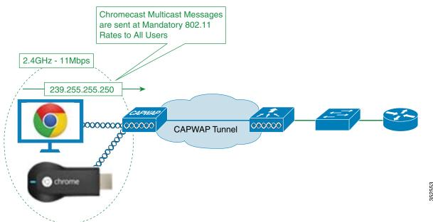
Multicast applications, such as Chromecast, require special consideration when being deployed over a wireless network because a multicast in 802.11 is sent out as a broadcast so that all clients can hear it. The actual data rate used by the AP in order to transmit the Chromecast frames is the highest mandatory rate configured within that band. For 2.4 GHz, the default rate is 11 Mbps.
