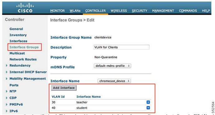
Step 3 (Optional: This can be achieved using a single interface as well, e.g. student). Go to the WLANs tab, and create the client SSID. Select the interface group created in Step 2.
