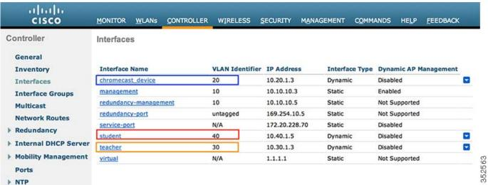
Step 2 (Optional: This can be achieved using a single interface as well). Go to the Controller tab > Interface Groups on the left-hand menu. Create a new interface group, and add the previously created client interfaces (teacher and student, in this example).
