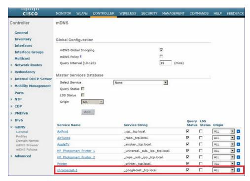
Now, you can add this service to the mDNS profile that is used on the WLAN. In this case, the default profile is used:
