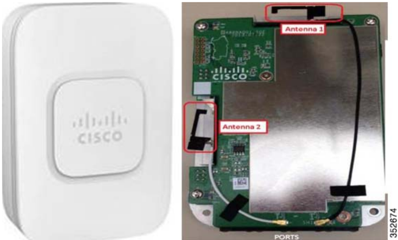
Figure 9 Antenna 1 and Antenna 2 mounted on the Top and Left Side of the AP-702W
