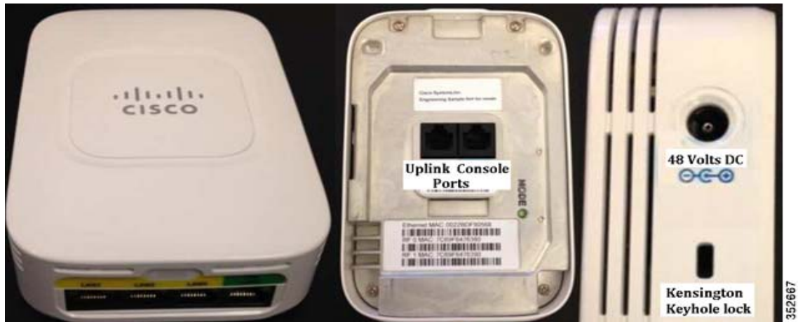
Figure 3 AP-702 Ethernet Switched Ports
