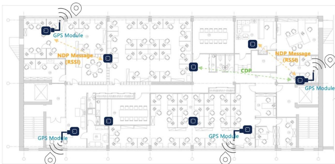
Figure 2. Geolocation Propagation Operation across an Indoor Floorplan
