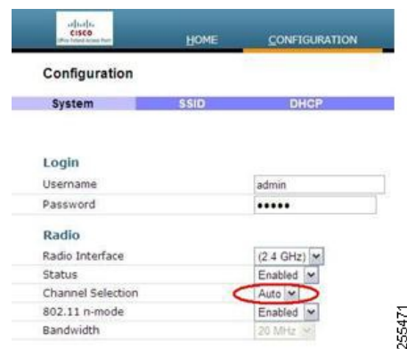
Figure 58: Channel Selection for OEAP 600 Series APs
