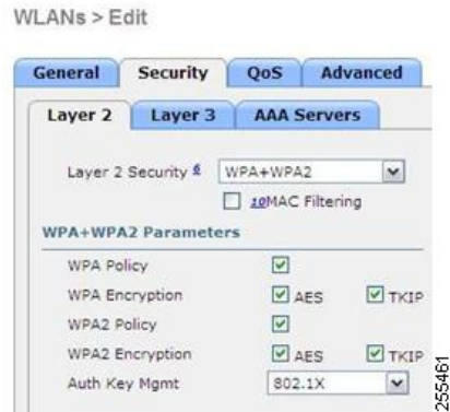
Figure 52: Compatible Security Settings for OEAP Series
