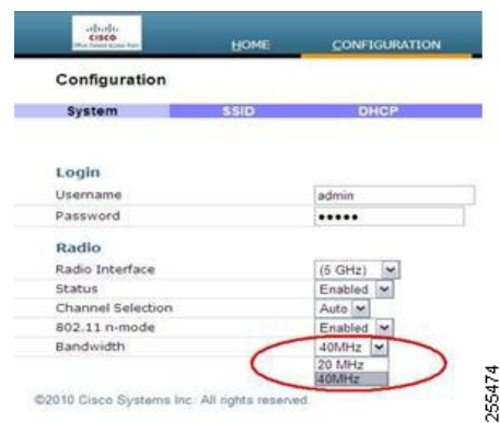
Figure 59: Channel Width for OEAP 600 APs
