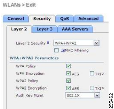
Figure 52: Compatible Security Settings for OEAP Series
