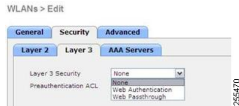
Figure 57: Layer 3 Security Settings for OEAP 600 Series APs in Remote LANs
