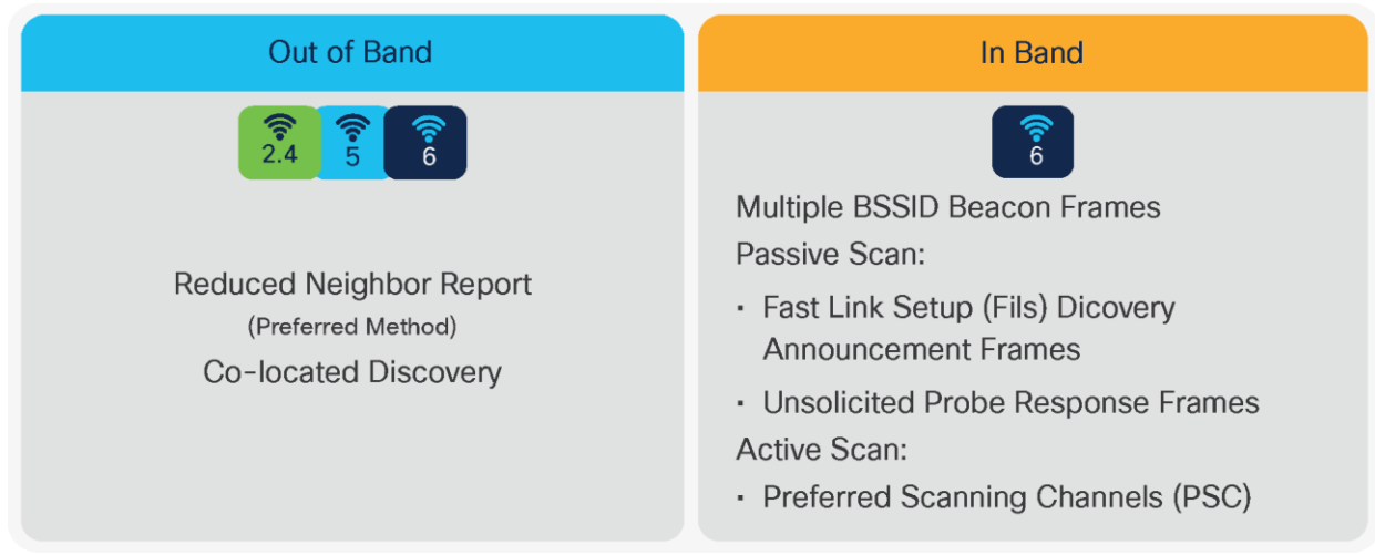
Figure 29. Out-of-band and in-band AP discovery mechanisms
