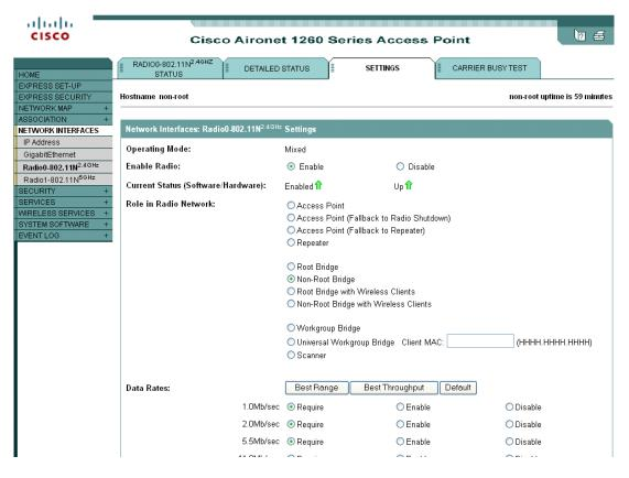
Figure 1 Network Interfaces: Radio Settings Page
