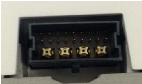
Figure 11 Smart Antenna Connector C9120AXE and C9120AXP Models
