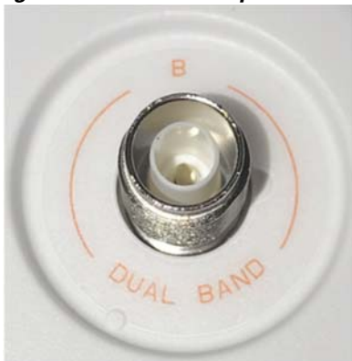
Figure 10 Dual-band port on C9120AXE and C9120AXP Models for non-Self-Identifying Antennas
