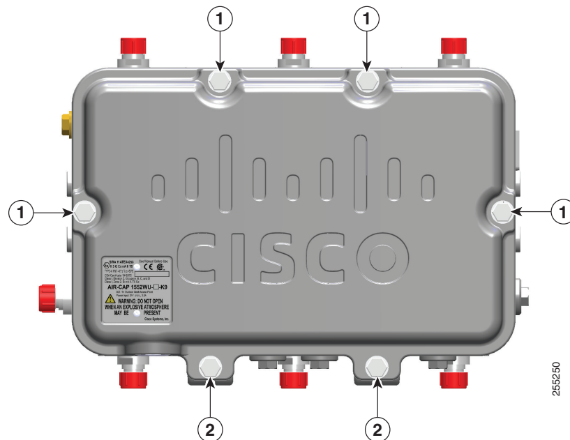
Figure 3-10 Access Point Front View of Hinged Cover
