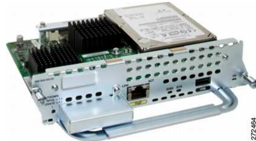
Figure 57 Cisco Unity Express Network Module
