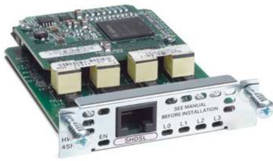
Figure 30 4-Port Symmetric High-Speed DSL (SHDSL) WAN Interface Card (HWIC-4SHDSL)
