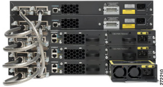
Figure 28 Catalyst 3750 in Cisco StackWise Configuration
