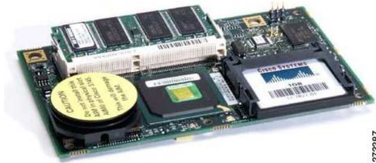
Figure 60 Cisco Unity Express Advanced Integration Module
