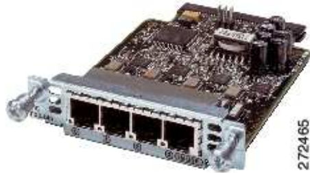
Figure 61 Four Port FXS/DID Voice Interface Card
