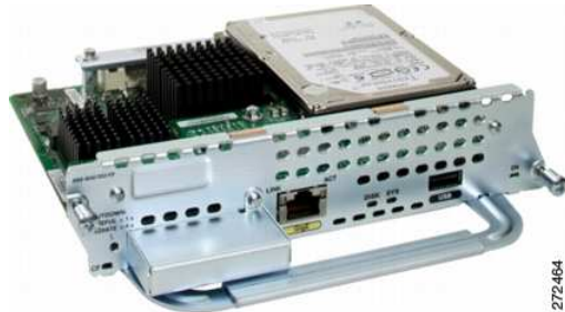
Figure 59 Cisco Unity Express Network Module
