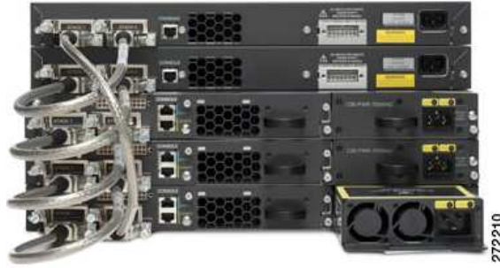
Figure 28 Catalyst 3750 in Cisco StackWise Configuration
