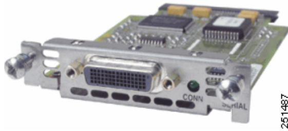
Figure 14 1-Port Serial High-Speed WAN Interface Card (HWIC-1T) with a T1 High-Speed Serial Port
