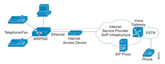
The WRP500 maintains the state of each call it terminates and reacts properly to user input events (such as on/off hook or hook flash). The WRP500 uses the Session Initiation Protocol (SIP) open standard, so little or no involvement by a "middle-man" server or media gateway controller occurs. SIP allows interoperation with all Internet telephony service providers (ITSPs) that support SIP.
