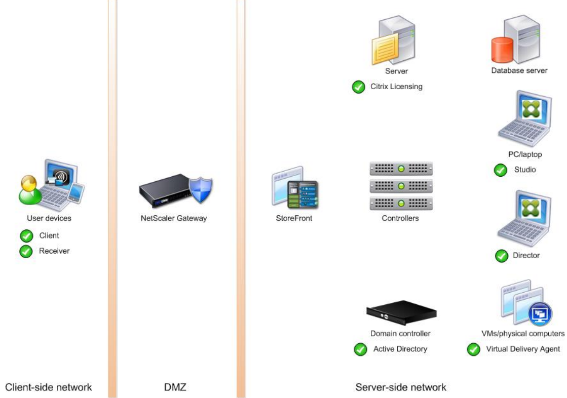
Figure 21 Example of a Distributed Components Configuration
