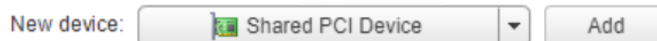
Figure 62 Adding a Shared PCI Device to the Virtual Machine to Attach the GPU Profile
