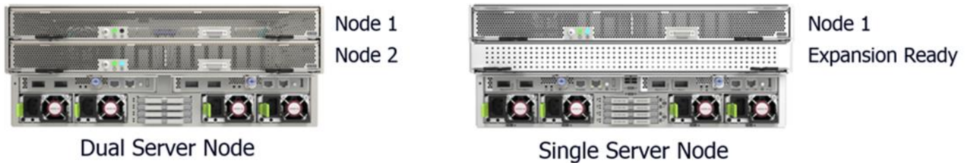
Figure 15 Single and Dual Node Rear Chassis View
