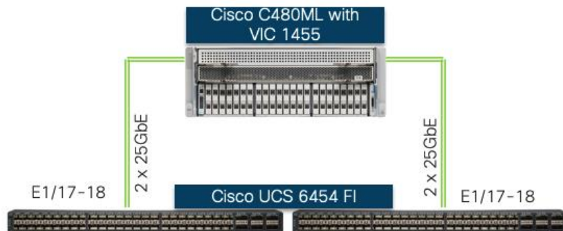
Figure 9 Cisco UCS C480 ML M5 to Cisco UCS 6454 FI Connectivity
