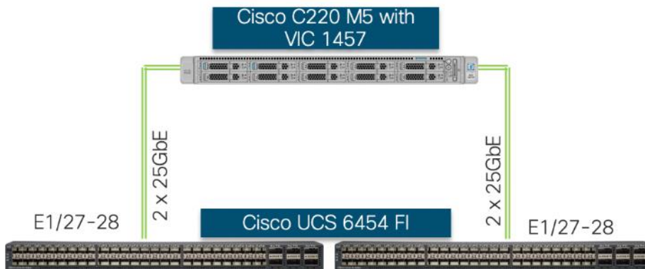
Figure 7 Cisco UCS C220 M5 to Cisco UCS 6454 FI Connectivity
