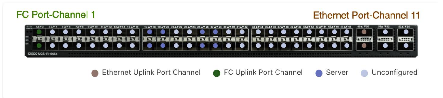
Figure 5. Cisco UCS Fabric Interconnect A port configuration
