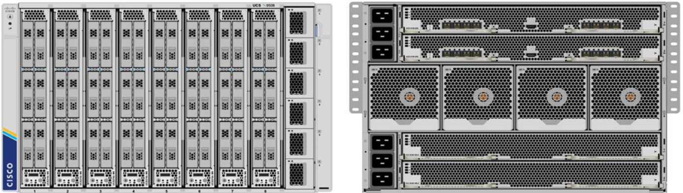
Figure 14. Cisco UCS X9508 Chassis front and rear view
