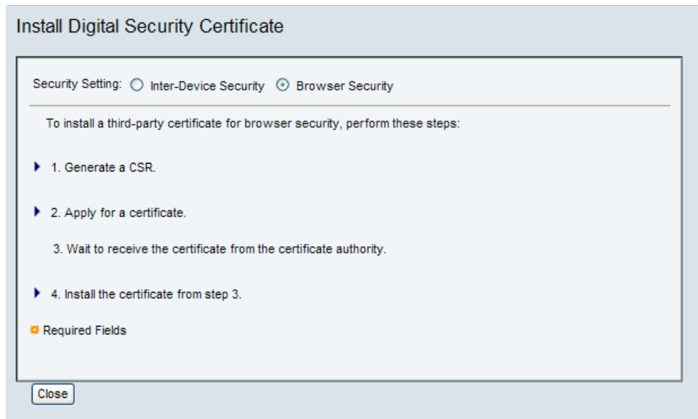
Figure 5-2 Install Digital Security Certificate Dialog Box—Browser Security Fields
