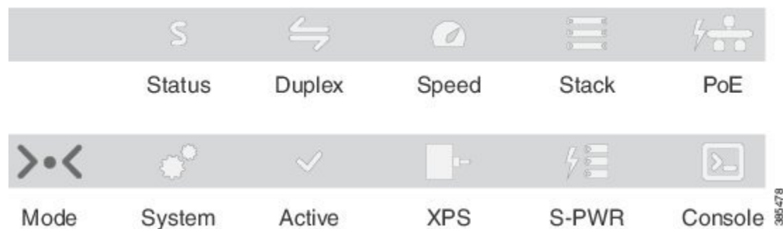
Figure 8: Switch Front Panel LEDs
