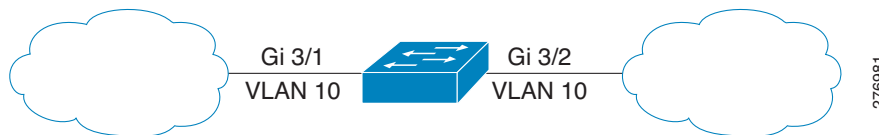
Figure 4-3 Disabling MAC Address Learning: Network Load Balancers
